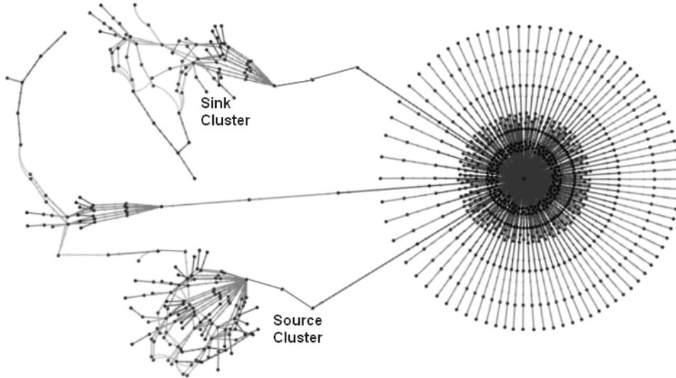
**Fig. 4.** Root-cause analysis of a source cluster with information flow to a sink cluster. The tree refinement derives only the sub-graphs relevant for an isolation breach. The “flower” is a large-scale switch.
